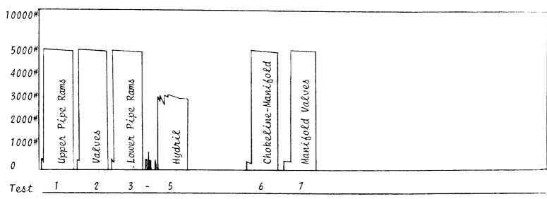
The above is a transposition of the pressure recorder chart covering test to the blowout control equipment in service on your well drilling in the Carlsbad, New Mexico Area, Midland District, Texas. Test was made with test plug landed in casing head with the following test results:
