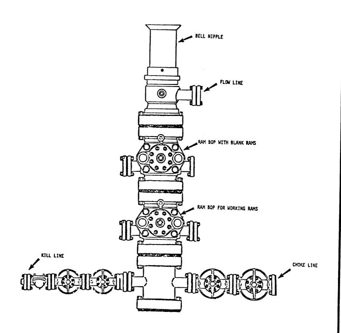
BOP rams will be actuated on each trip of drill pipe and will be tested before drilling the plug on each casing string.
