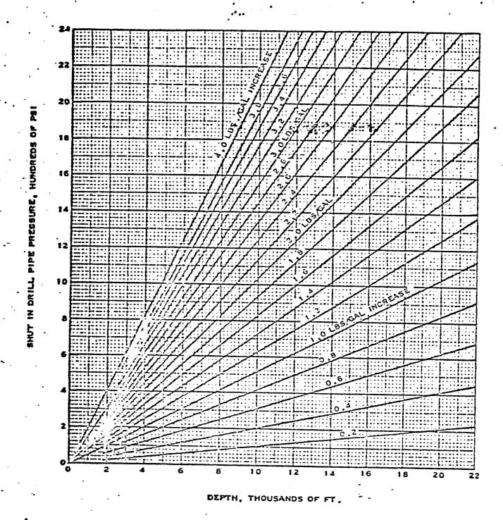
INCREASE IN MUD WEIGHT REQUIRED TO BALANCE FORMATION PRESSURE WHEN A DRILLING WELL IS SHUT IN AFTER A KICK
