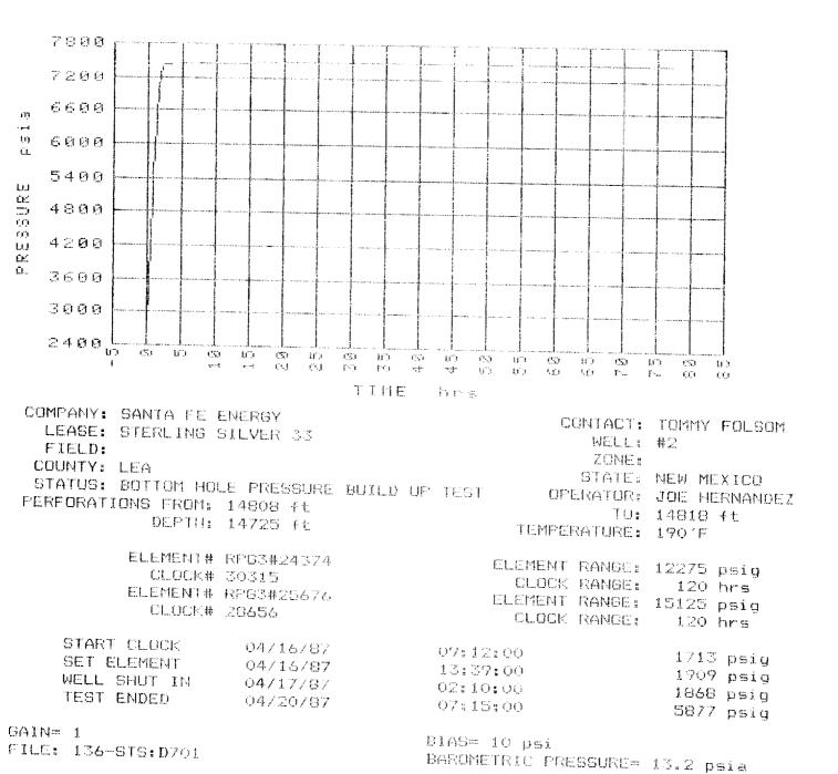
DURING THE FLOWING GRAIDENTS THE WELL WAS BEING FLOWED AT SUCH A RATE THAT THE PRESSURE READINGS WERE FALLING FASTER THAN COULD BE CORRECTLY MEASURED AT THE DEPTHS THAT WERE BEING MEASURED.
