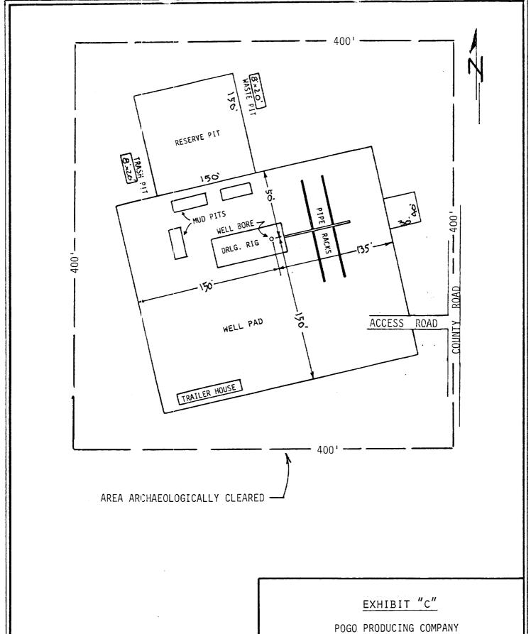
POGO PRODUCING COMPANY WELL NO.1 FEDERAL 26 DRILLING RIG LAYOUT SCALE: None
