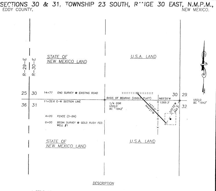
A STRIP OF LAND 50.0 FEET WIDE, 1477 FEET OR 0.280 MILES IN LENGTH AND BEING 25.0 FEET RIGHT AND 25.0 FEET LEFT OF THE ABOVE CENTERLINE SURVEY.
