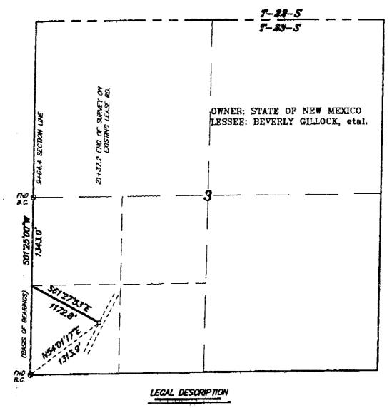
A SYRIP OF LAND 30.0 FEET HIDE, LOCATED IN SECTION 3, TOWNSHIP 23 SOUTH, RANGE 28 EAST, N.M.P.M., EDDY COUNTY, NEW MEXICO AND BEING 15.0 FEET LEFT AND RIGHT OF THE FOLLOWING DESCRIBED CENTERLINE SURVEY.
