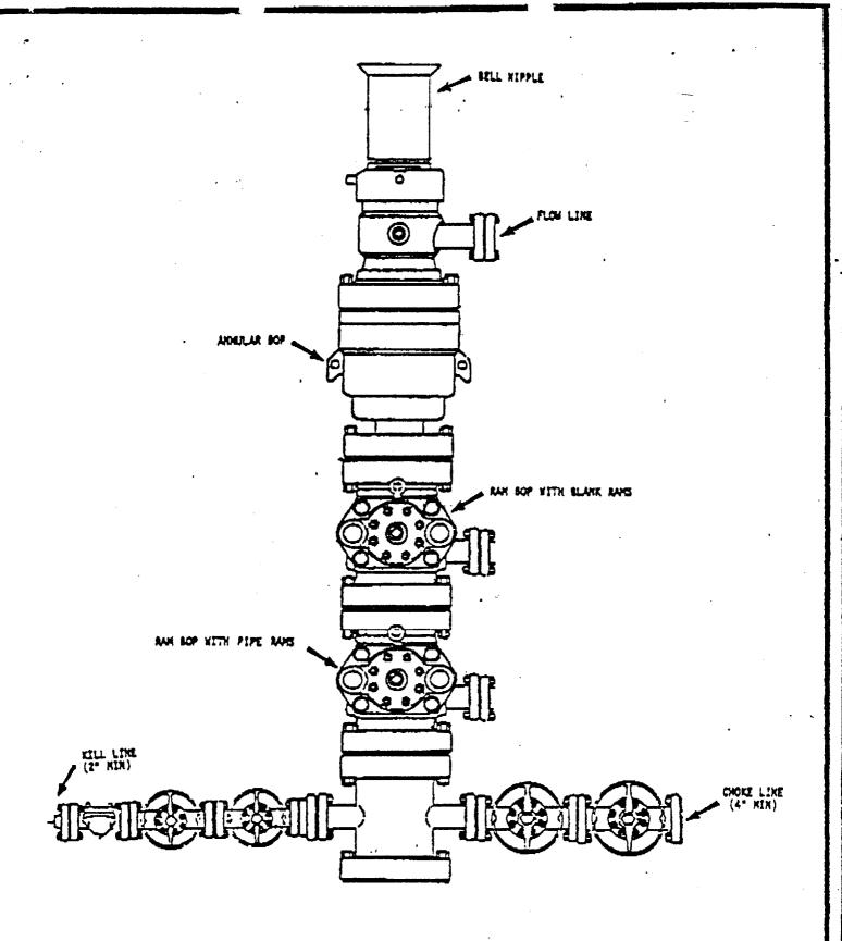
\*NOTE: ALL VALVES ARE METAL-TO-METAL SEAL AND FLANGED.
