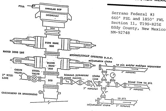
typical choke manifold assemby for 14 rated working pressure service-surface installation
