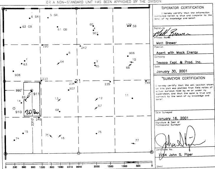
O = Staked Location • = Producing Well 💉 = Injection Well 💠 = Water Supply Well • Plugged & Abandon Well Equal Section Corner, 2 or 3" Iron Pipe & GLO B.C. = Found /4 Section Corner, 1" Iron Pipe & GLO B.C.
