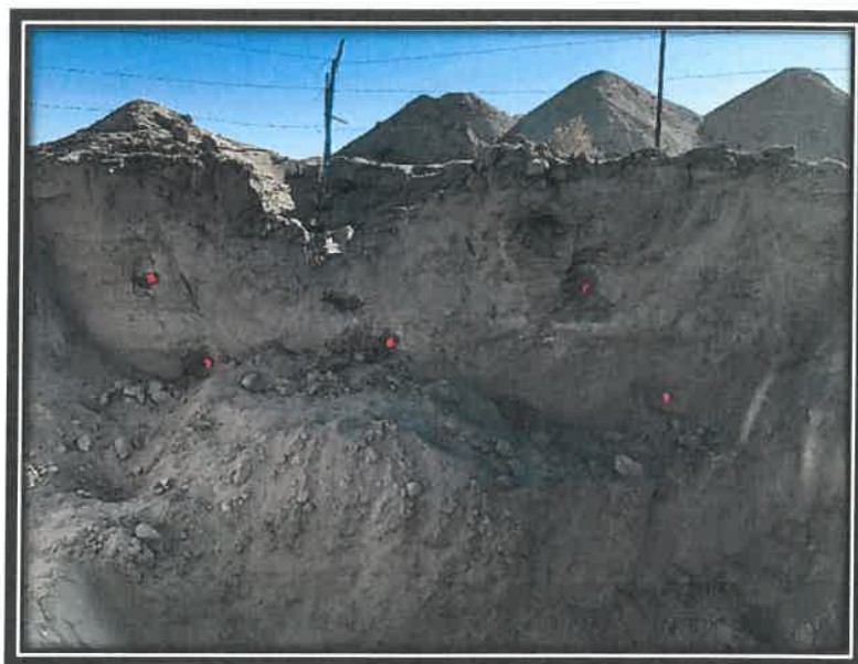
Picture 8: View of West Wall with Pin Flags (indicating sampling points)
