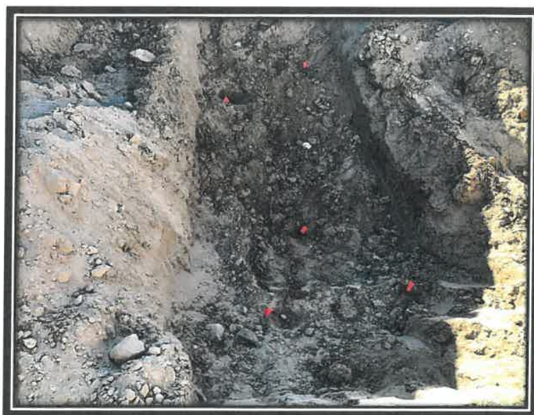
Picture 12: View of Base Center with Pin Flags (indicating sampling points)
