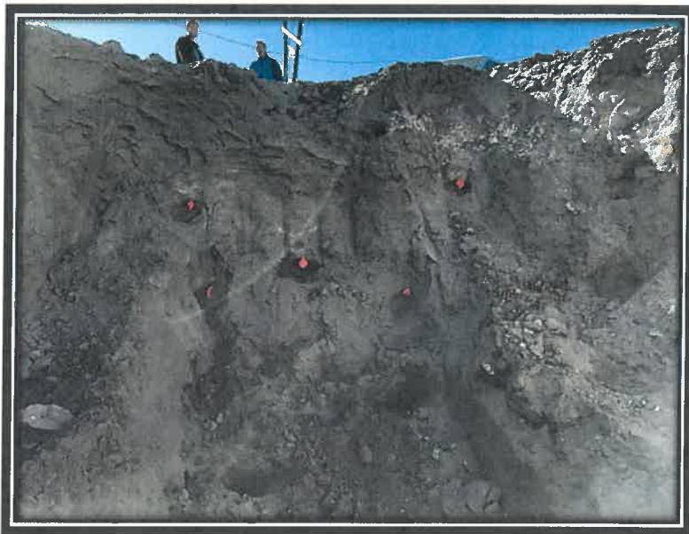
Picture 9: View of South Wall with Pin Flags (indicating sampling points)
