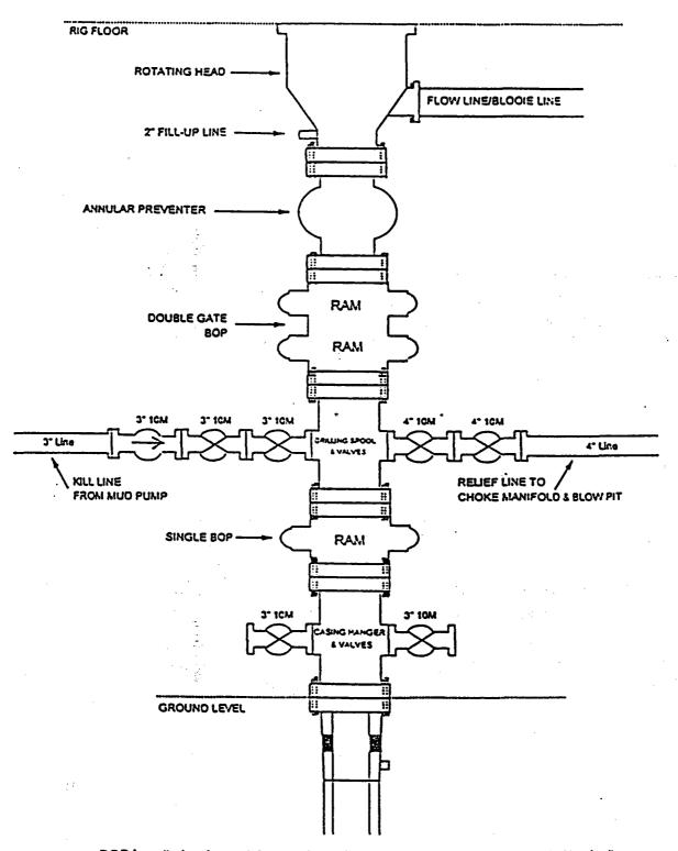
BOP installation from 13 3/8" casing point to TD. A 13 5/8" Bore (13 3/8" Nominal), 10,000 psi single gate BOP equipped with pipe rams will be installed on top of the casing hanger. A drilling spool will be installed on top of the single gate BOP. A 10,000 psi working pressure double gate BOP to be equipped with blind and pipe rams. A 5000 psi Annular preventer to be installed on top of the BOP. A rotating head to be installed on the top of the Annular preventer.
