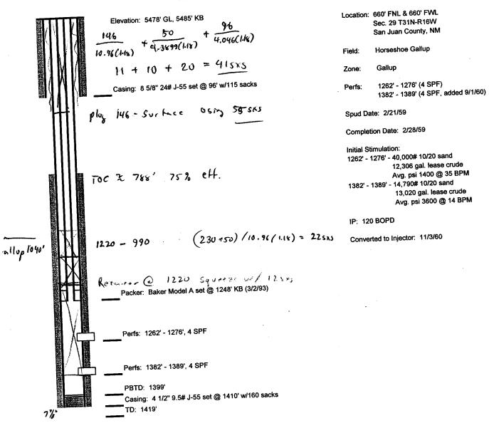
There are very few pulling reports on this well. The Lower Gallup was completed in 1960. In 1961 the well was acid treated. There are no reports of equipment failures prior to or after conversion. The well has been SI since 1986. When the casing was pressure tested in 1993, a large build-up of scale was found.
