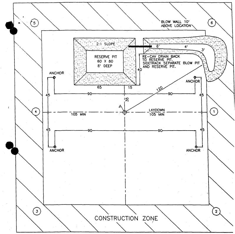
Blow pit averflow dike halfway between top and bottom and extend over plastic liner and into blow pit.
