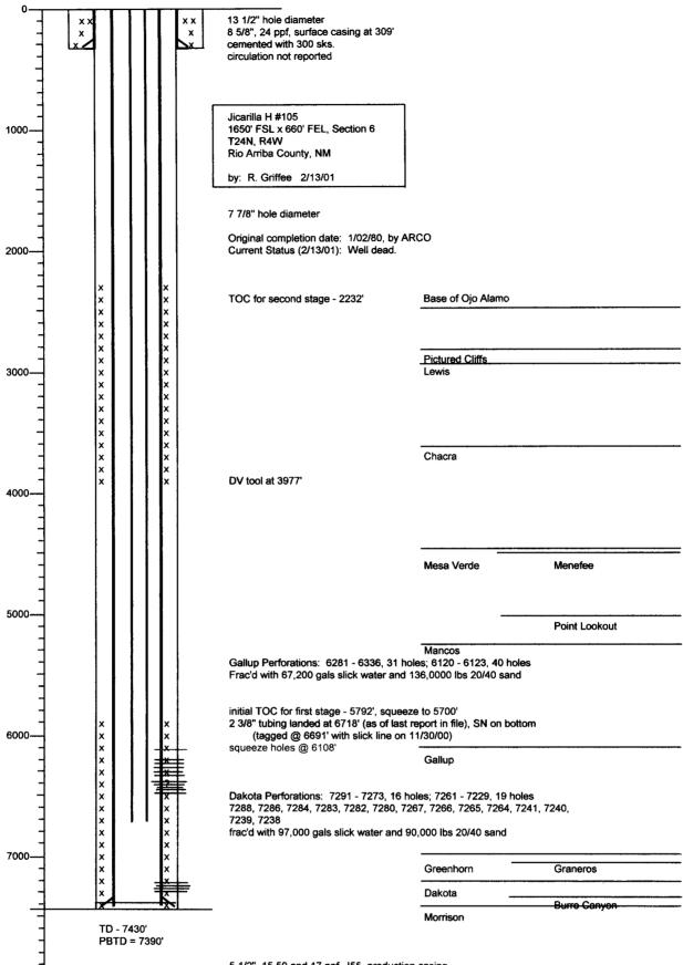
5 1/2", 15.50 and 17 ppf, J55, production casing set at 7429' (bottom 1316.51', 33 jts of casing is 17 ppf). Cemented with 650 sks in two stages
