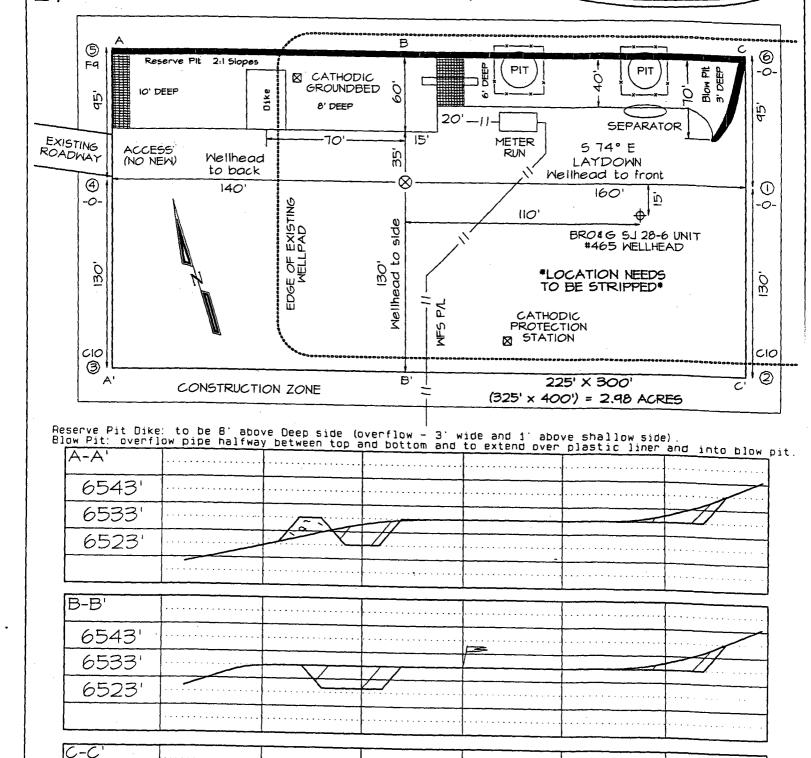
Note: Contractor should call One—Gall for location of any marked or unmarked buried pipelines or cable on well pad and/or access road at least two (2) working days prior to construction
