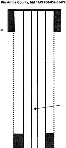
TD 6285' **PBTD 6172'**  9-5/8" Casing set @ 401' Cement with 200 sxs (Circulated to Surface)
