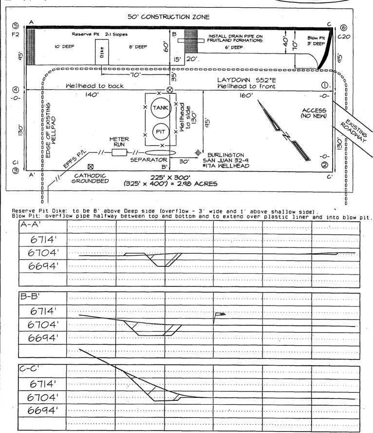
Note: Contractor should call One-Call for location of any marked or unmarked buried pipelines or cables on well pad and/or access road at least two (2) working days prior to construction
