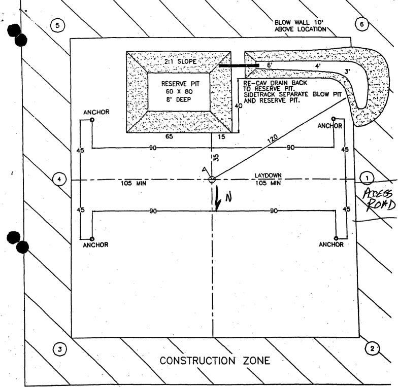
Blow pit overflow dike halfway between top and bottom and extend over plastic liner and into blow pit.
