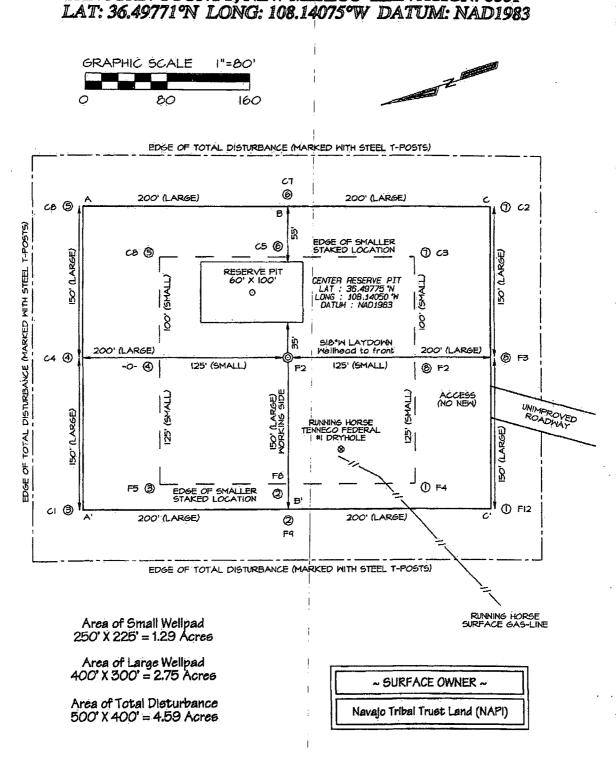
Steal T-Posts have been set to define the Edge of Disturbance limits which are 50 offset from the edge of the staked wellpad
