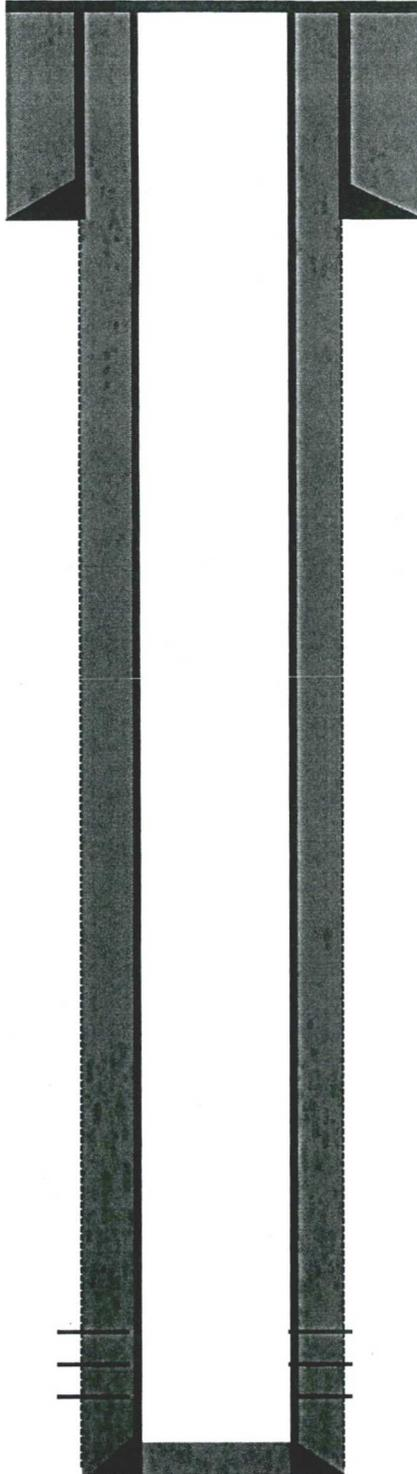
7-5/8" 26.4# casing @ 125'. Cemented with 125 sks Type III
