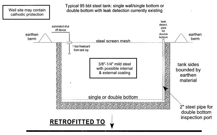
21/45/50 bbl steel tank: single wall/single bottom or double bottom with leak detection inserted into 95 bbl steel tank: single wall/single bottom or double bottom with leak detection/6" lift
