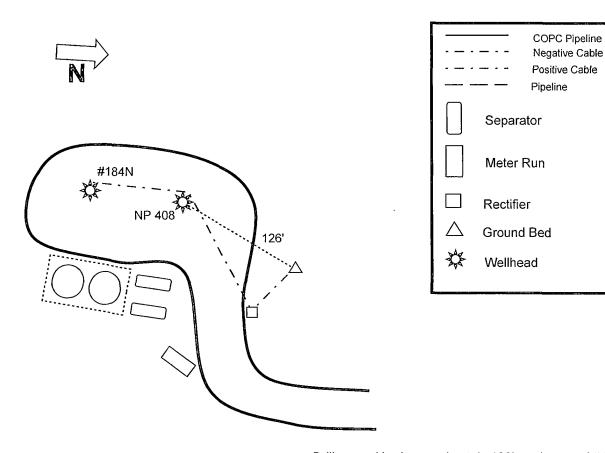
Drill ground bed approximately 126' north east of #408 wellhead at staked location. Install two well solar unit, and install cables to new ground bed and #184N and #408 wellheads at lengths below.
