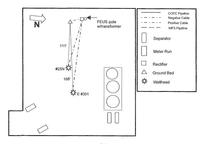
Drill ground bed approximately 111' west of #25N wellhead at staked location. Install 40-16 3 Negative rectifier on FEUS pole, and install cables to new ground bed and #25N and Howell E #301 wellheads at lengths below.
