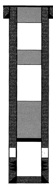
TD 4897' PBTD 4780' 9.625", 36#, J-55 Casing set @ 235' Cement with 150 sxs (Circulated to Surface)
