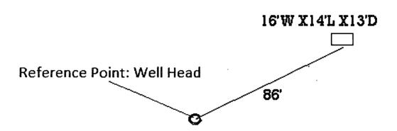
From Reference Point Go N. 40 Degrees NE. For a Distance of 86' to Center of Pit.
