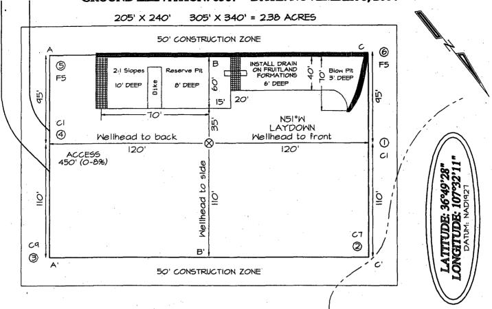
Reserve Pit Dike: to be 8' above Deep side (overflow - 3' wide and 1' above shallow side). Blow Pit: overflow pipe halfway between top and bottom and to extend over plastic liner and into blow pit.
