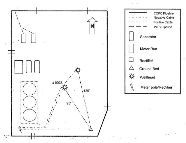
Drill ground bed approximately 93' South East of #100S wellhead at staked location. Install 40-16 3 negative rectifier unit on electric rack. Install cables to new ground bed and #100S wellhead at lengths below.
