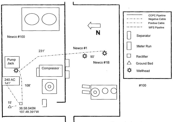
Drill ground bed on the Newco #100 location approximately 114' west of Newco #100 wellhead at staked location. Install 40-16 rectifier at staked location and connect to existing UGAC at pump master control panel. Install cable to new ground bed and to Newco #100, #1 and #1B wellheads at lengths below.
