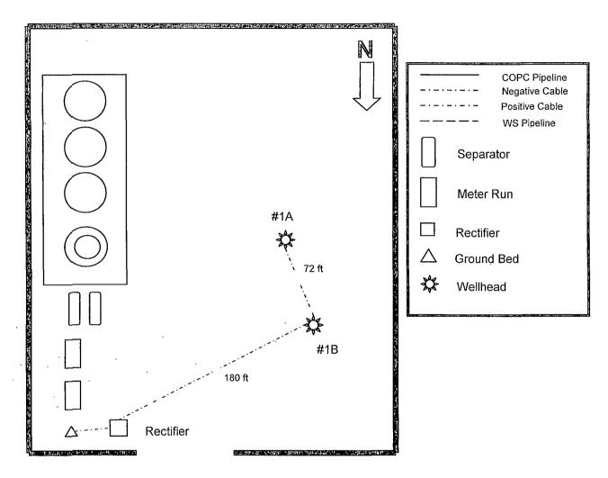
Drill ground bed approximately 177' North of #1B wellhead at staked location. Install new rectifier and cables to new ground bed, #1B and #1A wellheads. There is an existing ground bed, if possible tie in with new ground bed at rectifier. Tie in exsisting UGAC to new rectifier. Meterpole is on the outskirts of the location. The lengths of the new cables are listed below.
