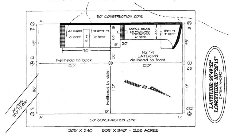
Reserve Pit Dike: to be 8' above Deep side (overflow - 3' wide and 1' above shallow side). Blow Pit: overflow pipe halfway between top and bottom and to extend over plastic liner and into blow pit.
