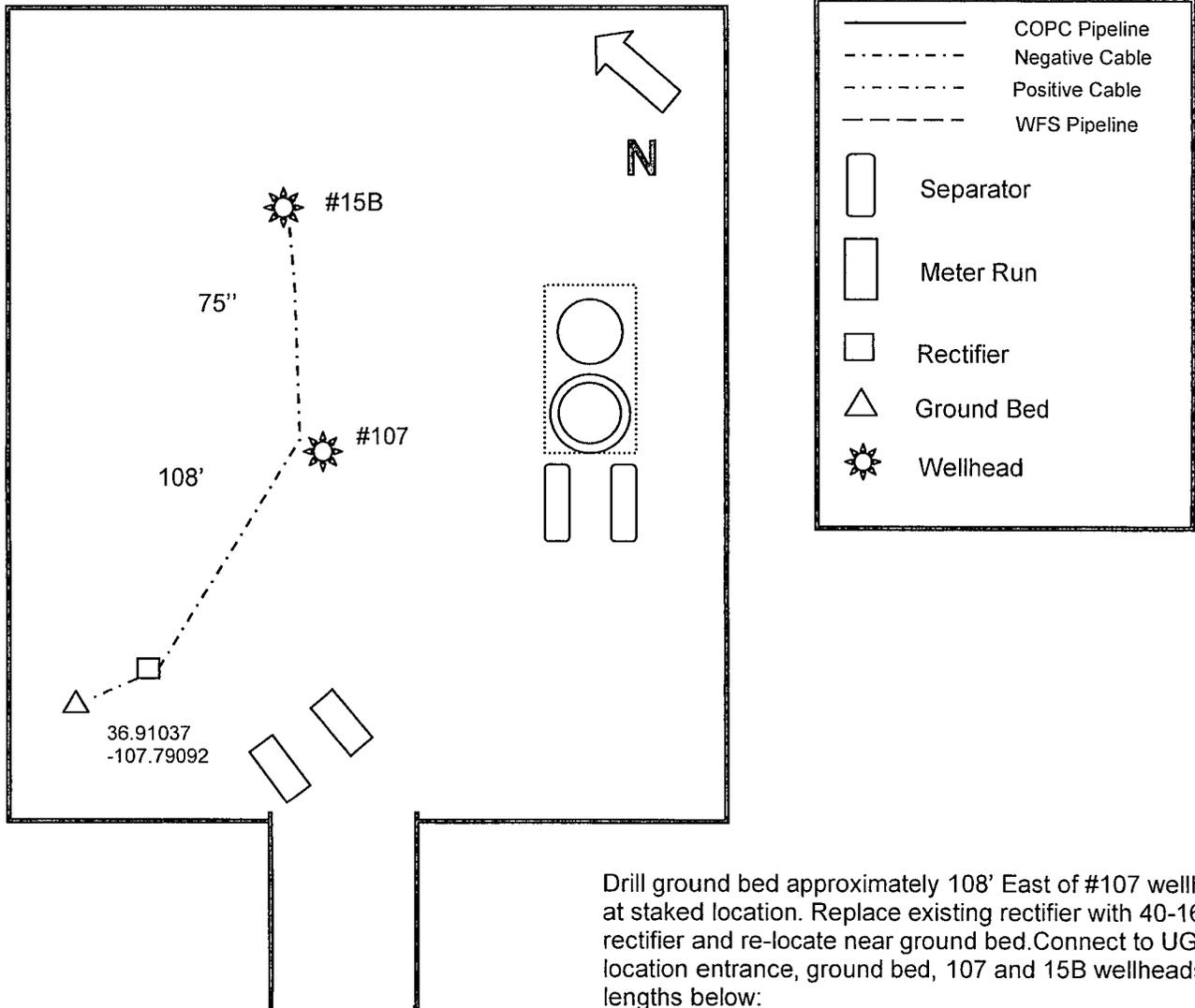
Drill ground bed approximately 108' East of #107 wellhead at staked location. Replace existing rectifier with 40-16 rectifier and re-locate near ground bed. Connect to UGAC at location entrance, ground bed, 107 and 15B wellheads at lengths below:
