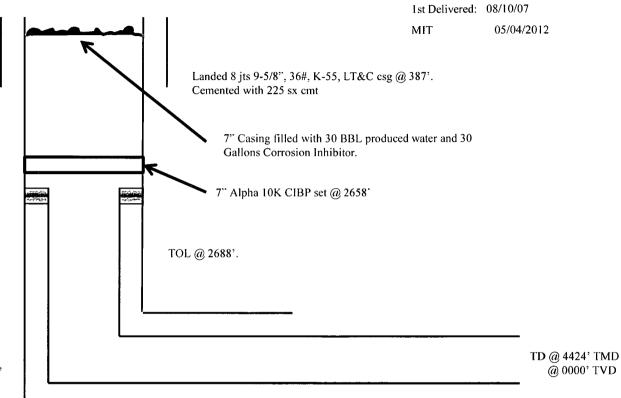
Hole Size Casing Cement Volume Top of CMT 225 sxs 12-1/4" 9-5/8",36# 215 cu.ft. surface 8-3/4" 7", 23# 700 sxs 1359 cu.ft. surface 6-1/4" 4-1/2",11.6# Did Not Cmt NΑ N/A
