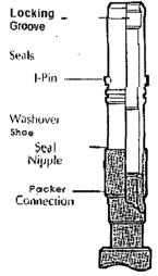
Baker HEL On-off tool-to unseat, PU rotate to the right (also made to rotate to the left) then set down.
