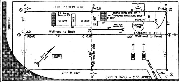
RESERVE PIT DIKE: TO BE 8' ABOVE DEEP SIDE (OVERFLOW - 3' WIDE AND 1' ABOVE SHALLOW SIDE). BLOW PIT: OVERFLOW PIPE HALFWAY BETWEEN TOP AND BOTTOM AND TO EXTEND OVER PLASTIC LINER AND INTO BLOW PIT.
