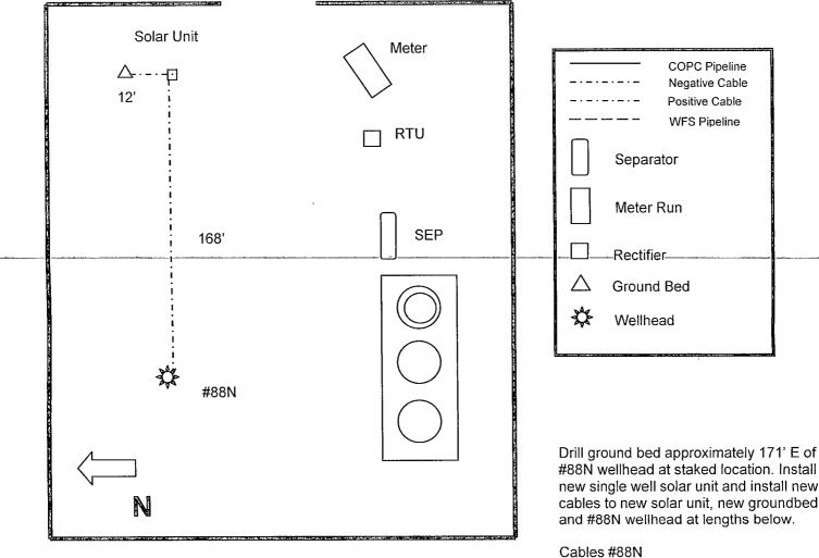
36 33.641' 107 45.307' #88N wellhead at staked location. Install new single well solar unit and install new cables to new solar unit, new groundbed
