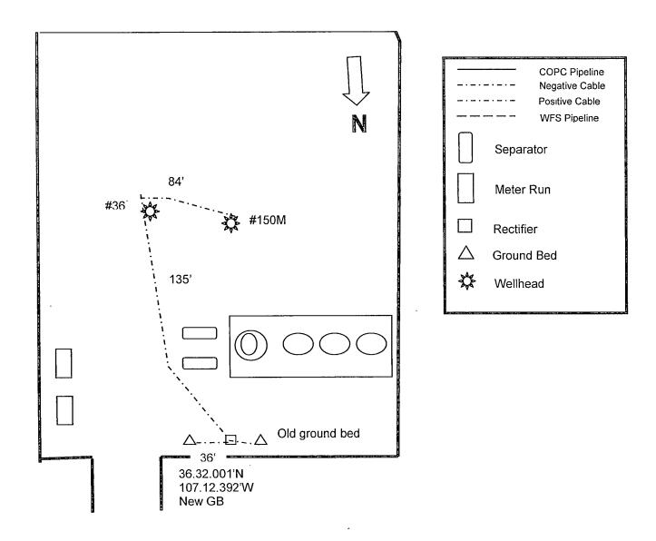
Drill ground bed approximately 135' north of #36 well head at staked location. Rectifier is already in place. Install cable to new ground bed and to #150M and #36 wellheads at lengths below.
