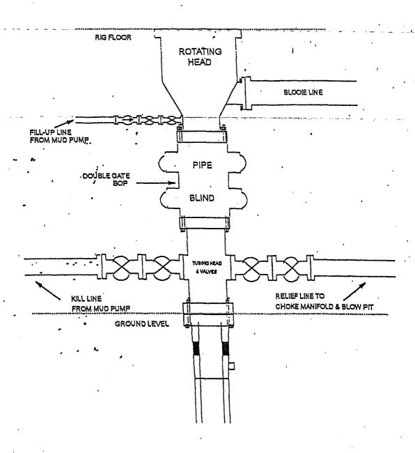
Minimum BOP installation for Completion operations. 7 1/16" Bore (6" Nominal), 3000 psi minimum working pressure double gate BOP to be equipped with blind and pipe rams.
