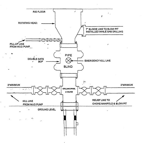
13 5/8" and 11" Bore, 2000psi minimum working pressure double gate BOP to be equipped with blind and pipe rams. A Schaffer Type 50 or equivalent rotating head to be installed on the top of the BOP. All equipment is 2000psi working pressure/ or greater.
