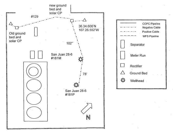
Drill ground bed approximately 105' north of #181M well head at staked location. Strip and upgrade existing single well solar to a duel well solar and reset at staked location. Install cable to new ground bed, old ground bed and to #181M and #181P well head's at lengths below.
