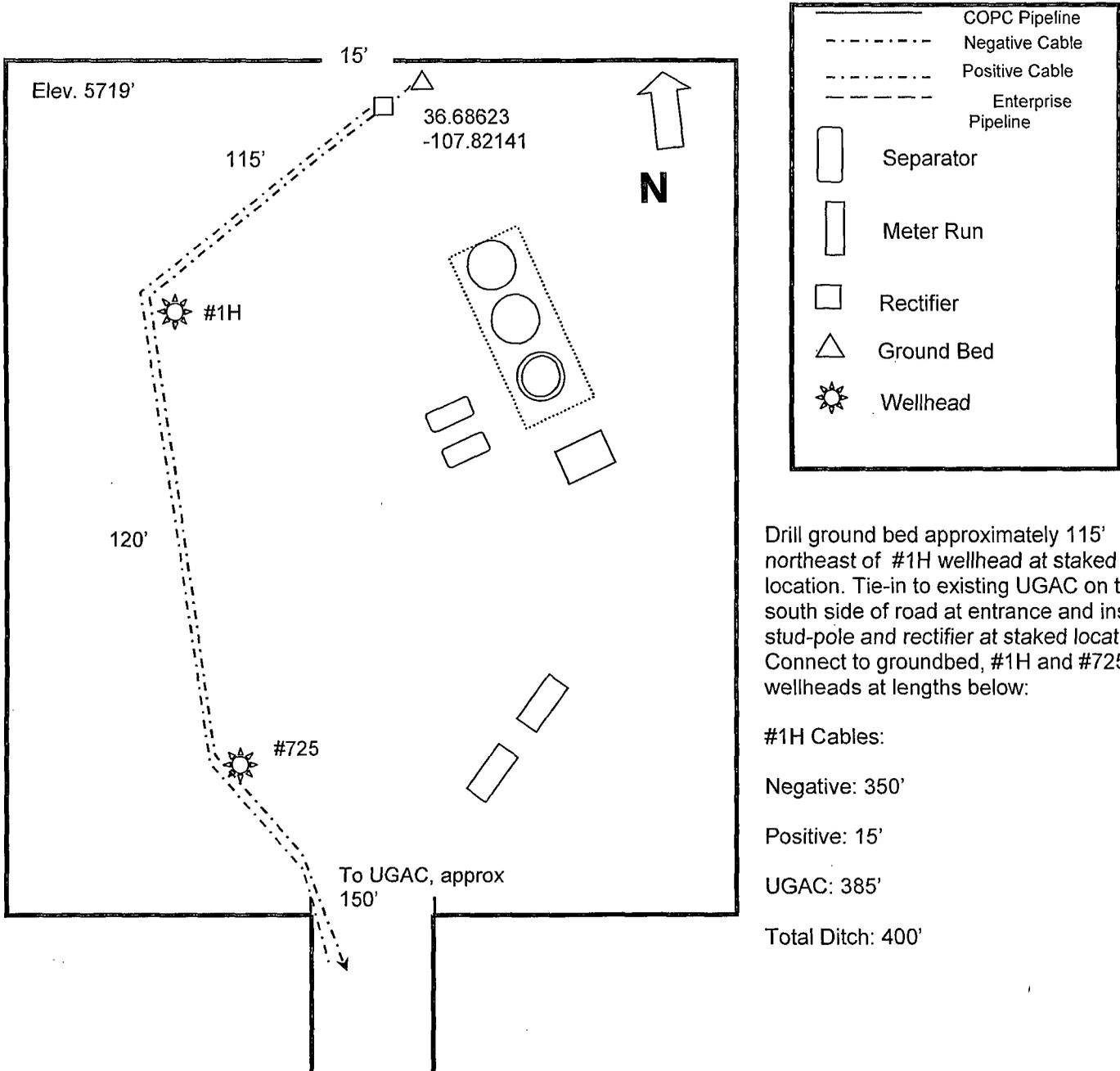
Drill ground bed approximately 115' northeast of #1H wellhead at staked location. Tie-in to existing UGAC on the south side of road at entrance and install stud-pole and rectifier at staked locations. Connect to groundbed, #1H and #725M wellheads at lengths below:
