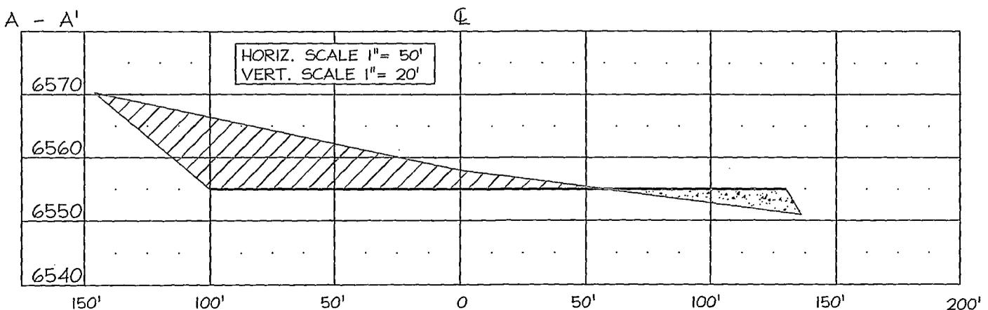
THIS DIAGRAM IS AN ESTIMATE OF DIRT BALANCE AND IS NOT INTENDED TO BE AN EXACT MEASURE OF VOLUME.
