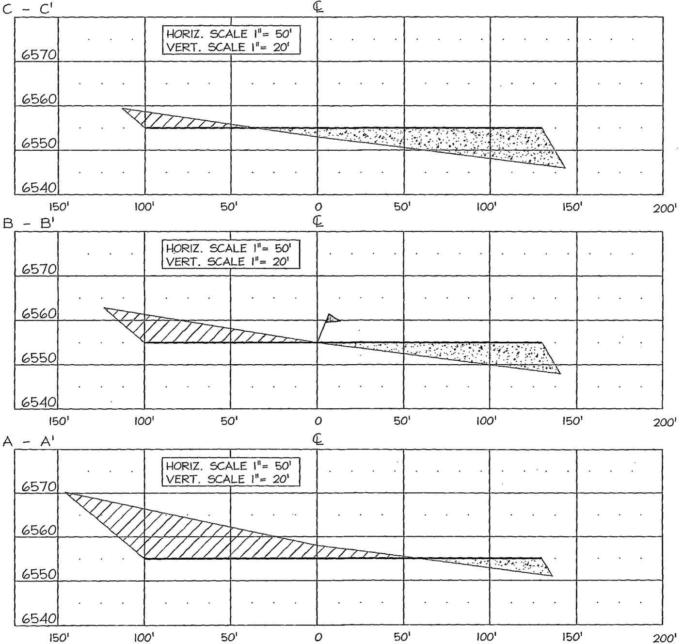
THIS DIAGRAM IS AN ESTIMATE OF DIRT BALANCE AND IS NOT INTENDED TO BE AN EXACT MEASURE OF VOLUME.
