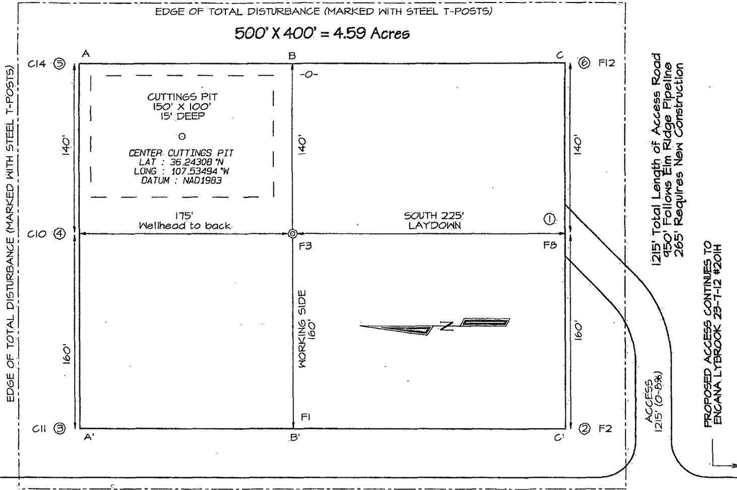
Steel T-Posts have been set to define the Edge of Disturbance limits which are 50' offset from the edge of the staked wellpad.
