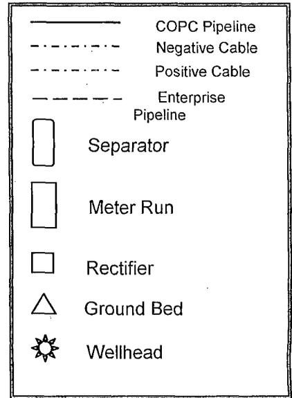
Drill ground bed approximately 120' southwest of #1N wellhead at staked location. Install solar unit at staked location and connect to #1N wellhead and ground bed at lengths below:
