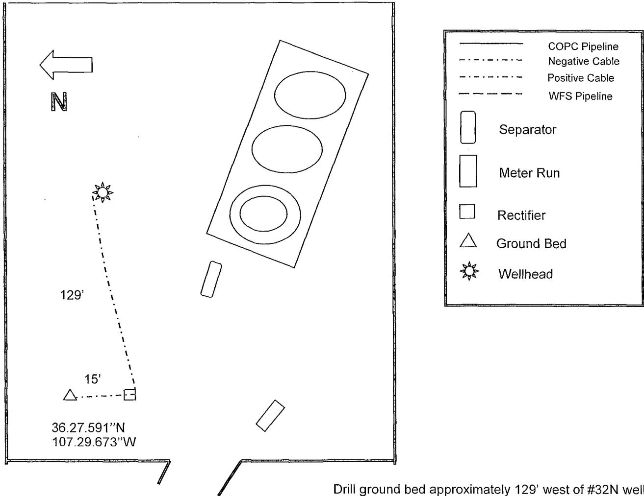
Drill ground bed approximately 129' west of #32N well head at staked location. Install single well solar at staked location. Install cable to new ground bed and to #32N well head at lengths below.
