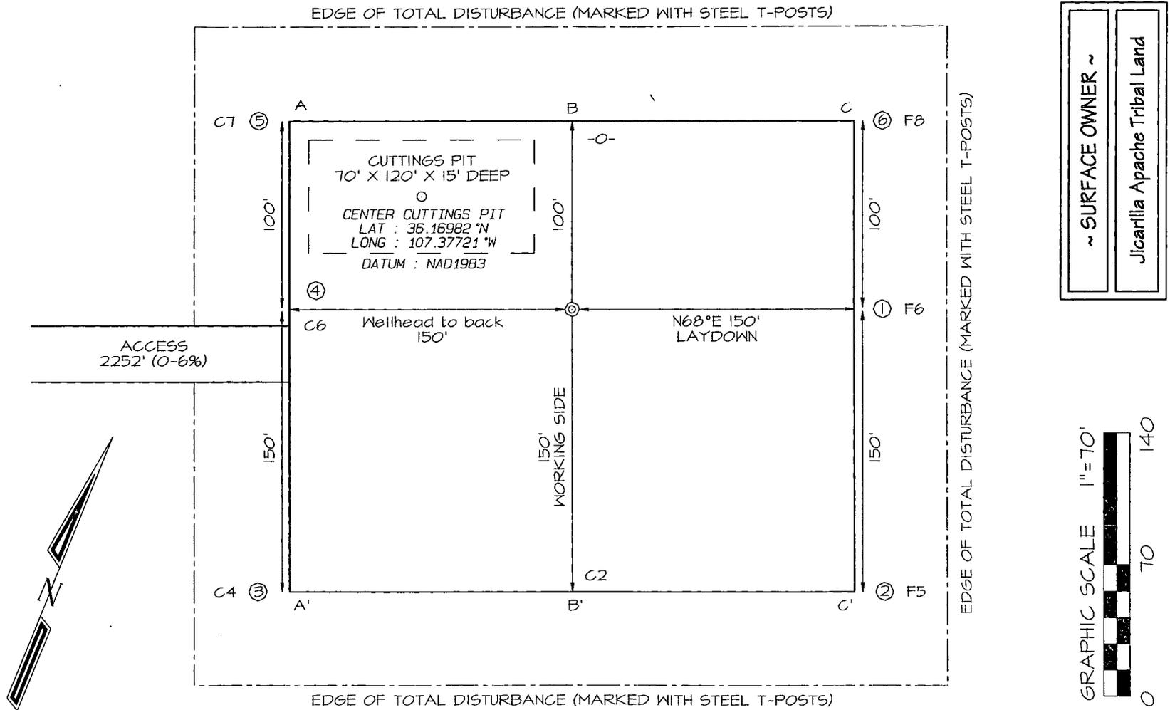
Steel T-Posts have been set to define Edge of Disturbance limits which are 50' offset from the edge of the staked wellpad.
