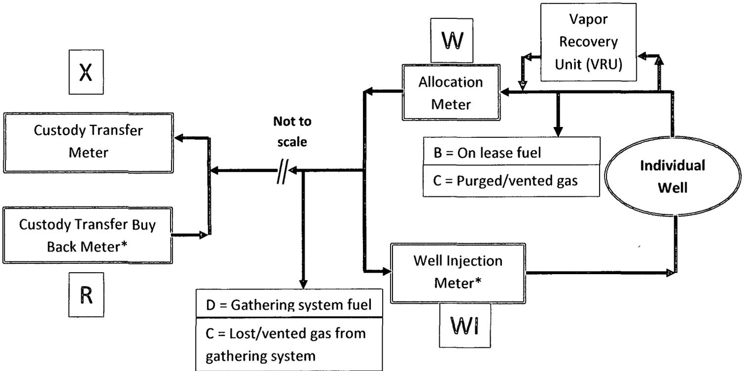
\*Meter will only be installed and active when gas lift is installed.
