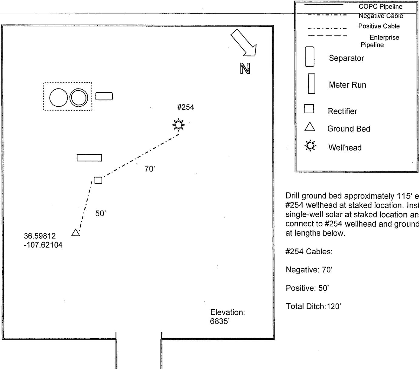
Drill ground bed approximately 115' east of #254 wellhead at staked location. Install single-well solar at staked location and connect to #254 wellhead and groundbed at lengths below.
