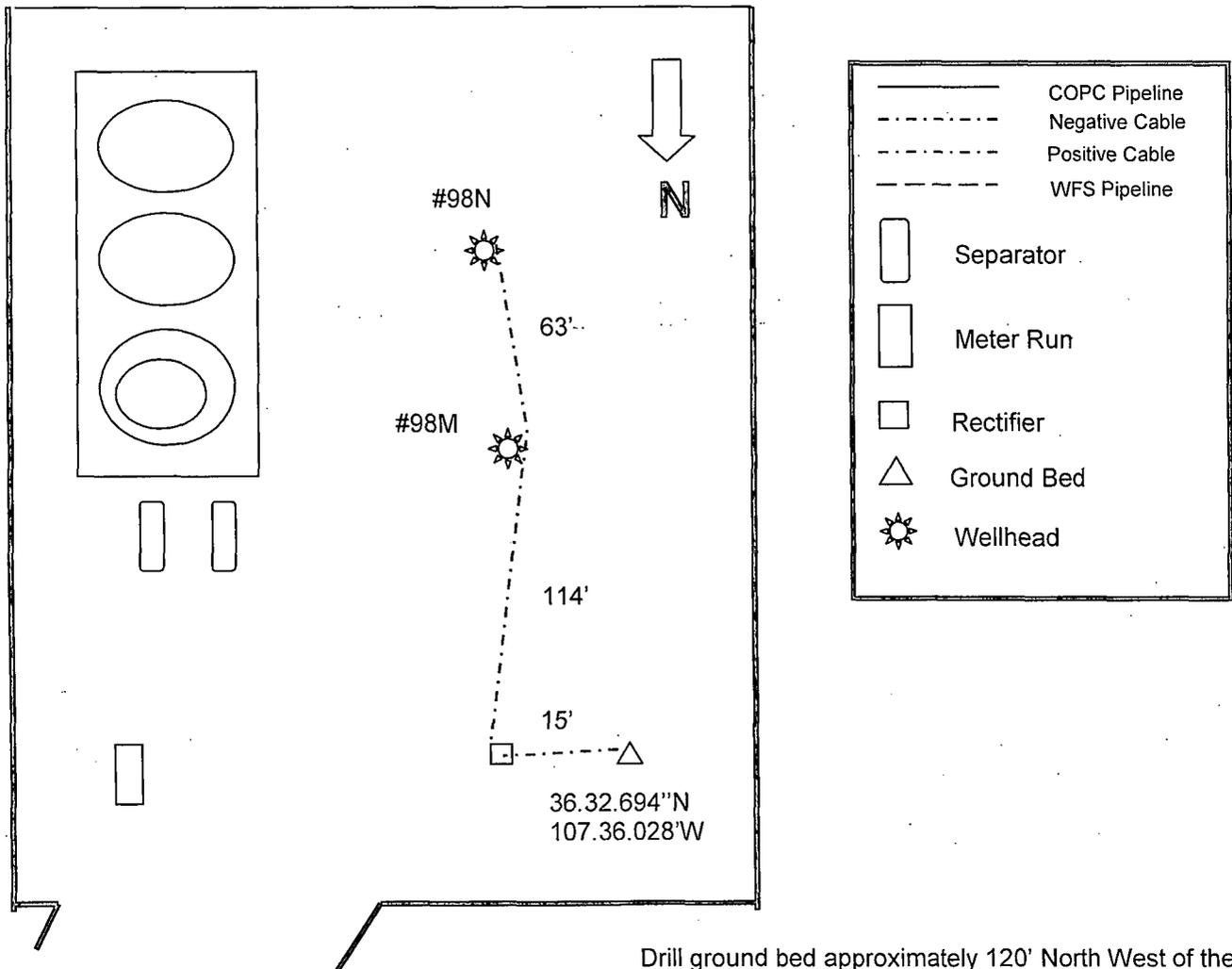
Drill ground bed approximately 120' North West of the #98M well head at staked location. Install a dual well solar CP at staked location. Install cable to new ground bed and to #98N and #98M wellheads at lengths below.
