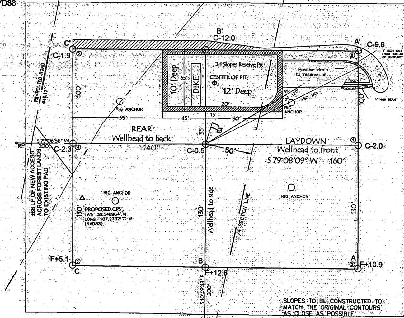
SLOPES TO BE CONSTRUCTED TO MATCH THE ORIGINAL CONTOURS AS CLOSE AS POSSIBLE
